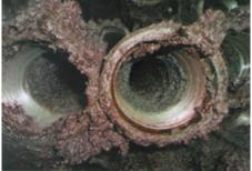
73mm diameter uncoated tubing
