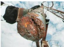
73mm diameter uncoated tubing removed from the well during workover
